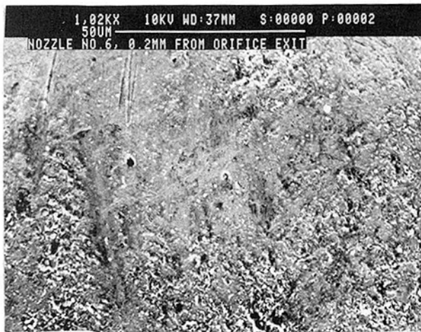
Fig. 7 High magnification photo of orifice surface after operation on low-ash CWS
